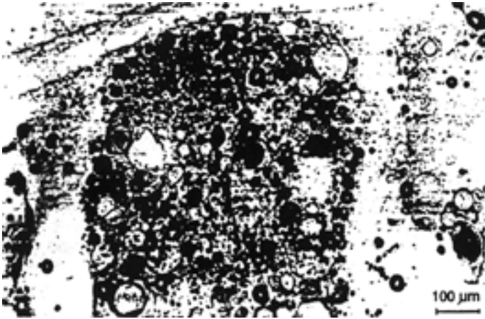
Figure 9: Small air bubbles in the cortex of a fulgurite, giving the lechatelierite matrix a foamy structure.
