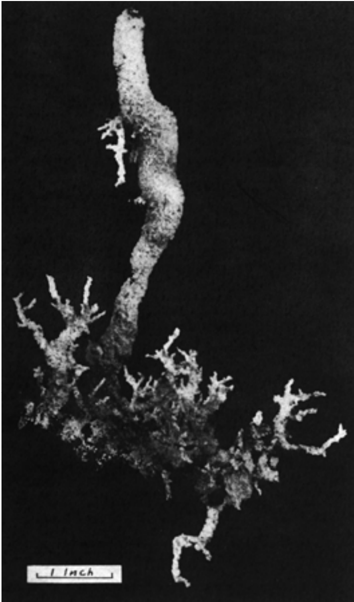
Figure 13: Artificial fulgurite made by passing electric current into grounded ten-quart pail of sand. (Courtesy General Electrical Company, Pittsfield, Mass.) (Petty, 1936, p. 197)
