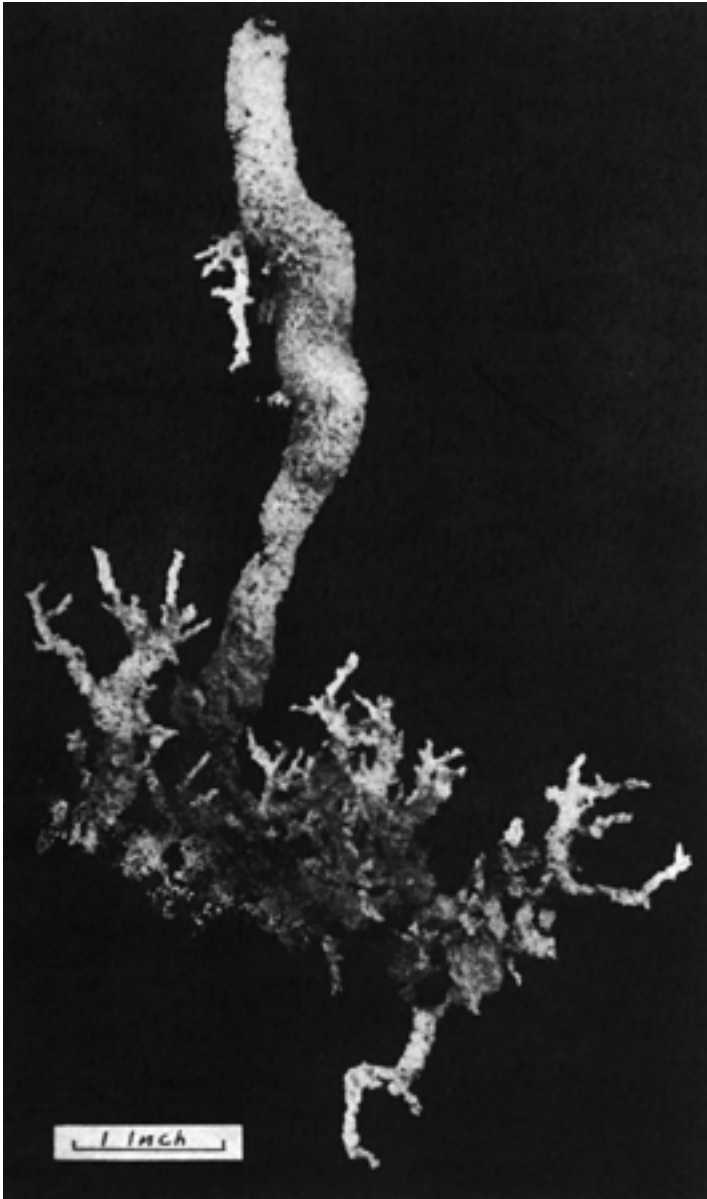
Figure 6: Artificial fulgurite made by passing electric current into grounded ten-quart pail of sand. (Courtesy General Electric Company, Pittsfield, Mass.)
